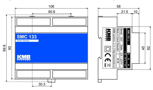
Figure 2: Dimensions of the SMC 133 analyzer.
