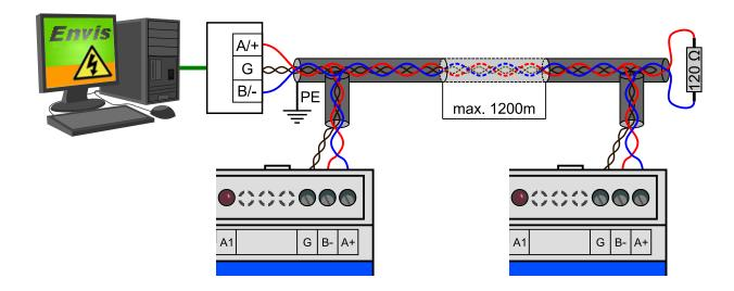
Figure 5: Typical wiring of the RS-485 communication line terminals in SMC 133.
