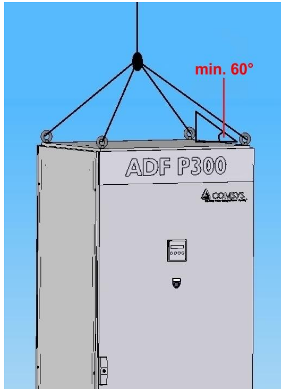
Figure 8: Correct lifting the Active Filter
