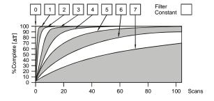
*Digital Filtering* module response to a temperature change. The illustration above demonstrates the effect of digital filtering (set with Filter Constant) on
