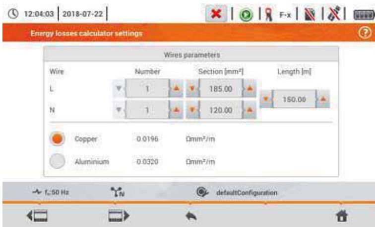
Fig. 5.29 Energy loss analysis – configuration screen 1
